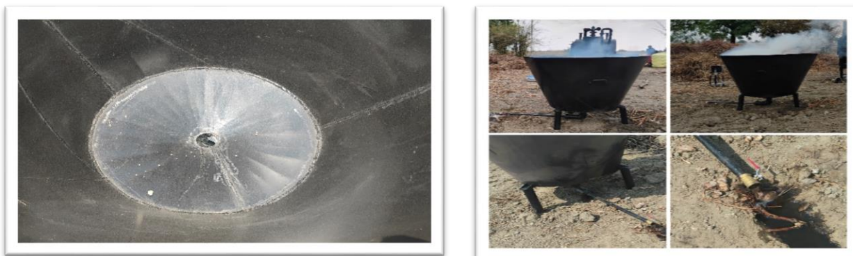
Fig. 6 Small tube attachments at the bottom of Kon-tiki to drain out excess water
