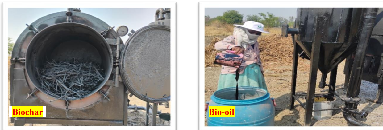
Fig. 7. Biochar production by furnace- pyrolysis machine
