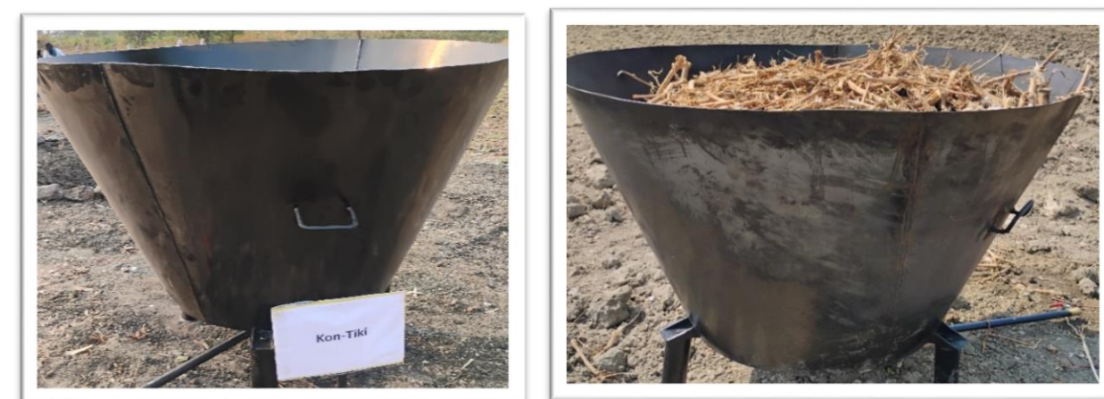
Fig. 5 Modified Kon-Tiki pyrolysis Kiln
